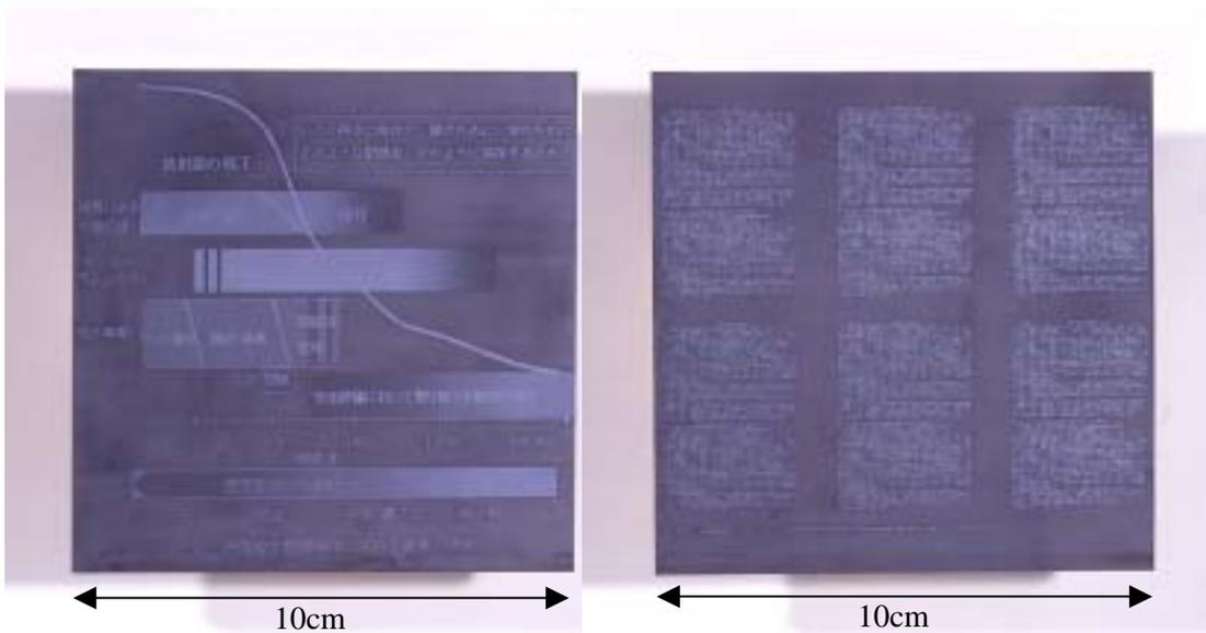
Fig. 6-6. Figures and Scaled Down Sentences Engraved on Silicon Carbide (Sintered Compact)
