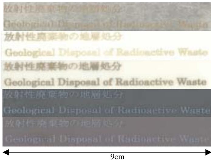
From above to bottom, hastelloy, alumina, zirconia, silicon carbide sintered compact, and silicon carbide (CVD). The size of character is 11 point
