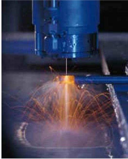
Fig. 6-1 Laser/Water Jet Hybrid Machining
