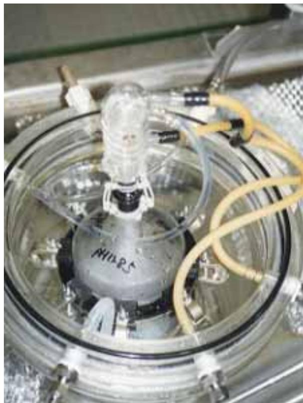
Fig. 3.2-7 Schematic representation of test vessel and photo showing the interior
