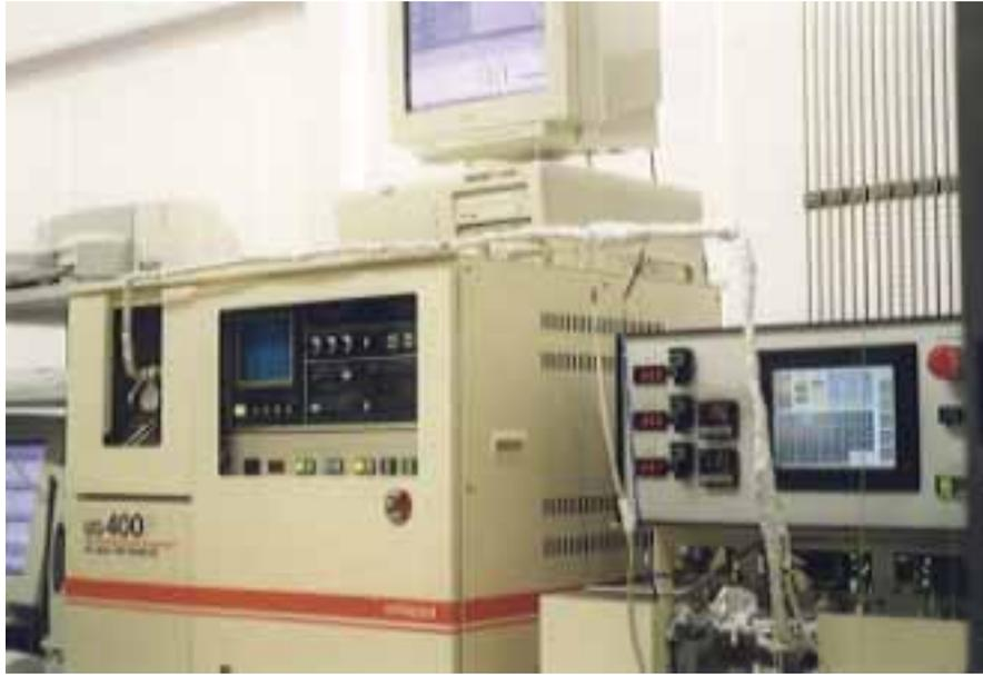
Atmospheric pressure ionization mass spectrometer (APIMS)
