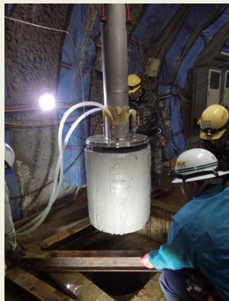
State of the specimen after bentonite erosion test at the URL
