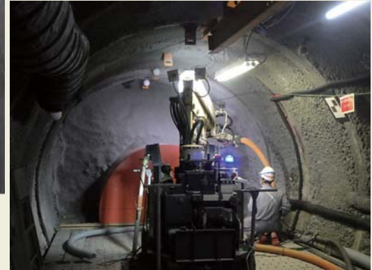
Backfilling test by spraying method
