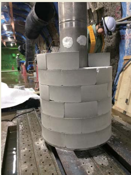
Specimen for bentonite erosion test of buffer material at the underground research laboratory (URL)
