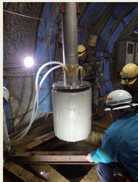
State of the specimen after bentonite erosion test at the URL
